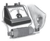
An electric current is induced when you move a magnet through a coil of wire.
