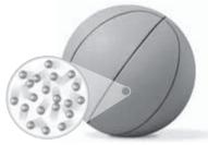
The basketball has a higher pressure because there are more particles of gas in it, and they are closer together. The particles collide with the inside of the ball at a faster rate.
