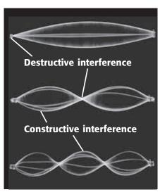
A rope vibrating at certain frequencies can create a standing wave. The initial wave travels down the rope and will be reflected back when it reaches the end. In a standing wave, certain parts of the wave are always at the rest position. This point is caused by destructive interference between the waves. Constructive interference can be seen at points in the wave where there is large amplitude.
