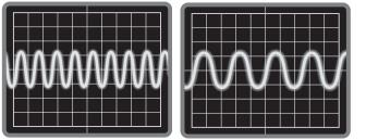
The wave in the graph on the right has a lower frequency than the one on the left. Therefore, the sound represented by the right-hand graph has a lower pitch than the one represented on the left.
