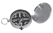
The needle in a compass is a magnet that is free to rotate.
