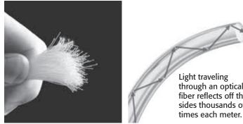
Light traveling through an optical fiber reflects off the sides thousands of
