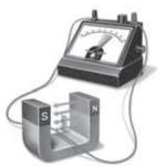
As the wire moves between the poles of the magnet, it cuts through magnetic field lines. This induces an electric current.
