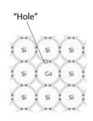
P-Type Semiconductor An atom of gallium, Ga, has three electrons in its outermost energy level. Replacing a silicon atom with a gallium atom results in a "hole" where an electron could be.
