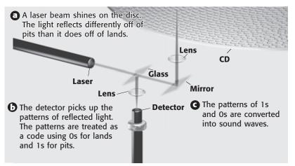
Different sequences and sizes of pits and lands will register different patterns of numbers that are converted into different sounds.
