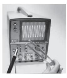
A receiver on an oscilloscope converts a sound wave into an electrical signal. The signal travels to a computer in the oscilloscope. The computer interprets and graphs the sound wave as a transverse wave.
