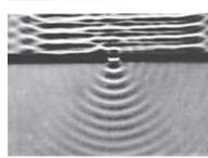
If the barrier or opening is the same size or smaller than the wavelength of an approaching wave, the amount of diffraction is large.
