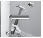
A hammer is an example of a thirdclass lever. Third-class levers have a mechanical advantage that is less than 1. The output force is less than the input force. Third-class levers increase the distance that the output force acts on.
