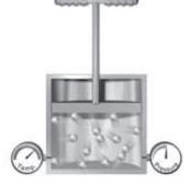
Increasing the temperature of a gas makes the particles move more quickly. The gas particles hit the piston more often and with more force. Therefore, the volume of the gas increases.
