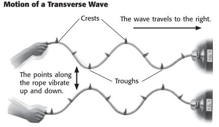
A wave traveling down a length of rope is an example of a transverse wave. The wave travels to the right. The particles in the medium, the rope, travel up-and-down. The particles in the wave and the medium are moving at right angles to each other.
