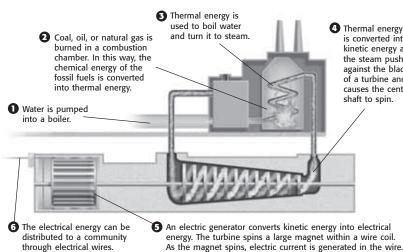
is converted into kinetic energy as the steam pushes against the blades of a turbine and causes the central
