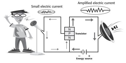
• Sound waves from your voice enter the microphone. As a result, a small electric current is made in the microphone side of the circuit. • A transistor allows the small electric current to control a larger electric current that operates the loudspeaker. The current in the loudspeaker is larger than the current produced by the microphone. Otherwise, the two currents are identical.
