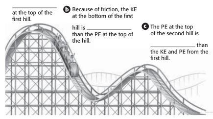
Not all of the cars' potential energy (PE) changes into kinetic energy (KE) as the cars go down the first hill. When the cars move up hill 2, not all of its KE is converted into PE at the top of hill 2. Some of it is changed into thermal energy because of friction.
