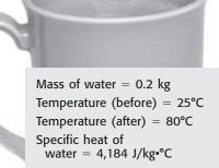
Information used to calculate heat, the amount of energy transferred to the water, is shown here.
