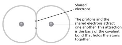
By sharing electrons in a covalent bond, each hydrogen atom (the smallest atom) has a full outermost energy level containing two electrons.
