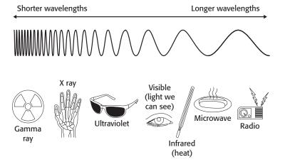
The electromagnetic spectrum is arranged from short to long wavelength. This is the same as arranging from high to low frequency.
