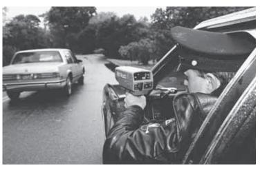
Police officers often use radar to detect the speed of a car. The radar gun is used to determine whether a car is traveling faster than the speed limit.
