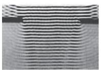
If the barrier or opening is larger than the wavelength of the wave, there is only a small amount of diffraction.
