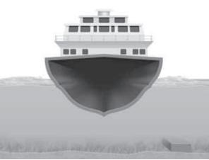
A block of steel is denser than water, so it sinks. If that block is shaped into a hollow form, the overall density of the form is less than water. Therefore, the ship floats.
