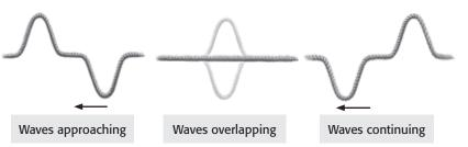
**Destructive Interference** When two waves with the same amplitude combine by destructive interference, they cancel each other out.
