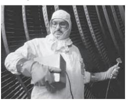
Tracers are used to find weak spots in materials and leaks in pipes. A Geiger counter is often used to detect the tracer.
