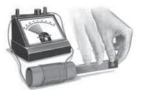
**O** The induced electric current reverses es direction if the magnet is pulled out rather than pushed in.
