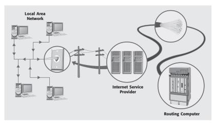
Modems, cables, phone lines, and fiber optic cables link computers around the world. Internet Service Providers allow small computers to connect to large routing computers. People can use browsers to access the World Wide Web. They can use other software to access other parts of the Internet.
