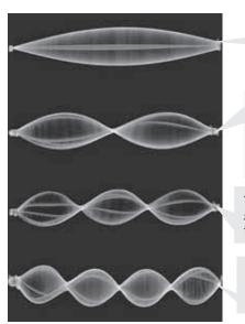
This string vibrates in only one standing wave. The frequency of the sound the string produces is the fundamental frequency.
