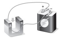
Switching the wires at the battery reverses the direction of the electric current. Now the wire will be pushed down.
