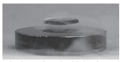
One interesting property of superconductors is that they repel magnets. The superconductor in this photograph is repelling the magnet so strongly that the magnet is floating.
