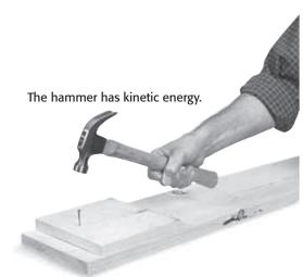
When you swing a hammer, it is moving. It has kinetic energy. This energy does work on the nail driving it into the wood.
