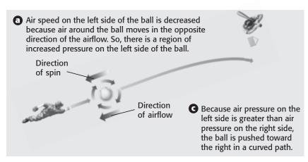
The picture above shows how a baseball pitcher can use Bernoulli's principle to throw a confusing screwball. It is hard for a batter to hit.
