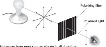
Light waves from most sources vibrate in all directions. Polarizing filters have long molecules that line up like parallel slits. Light waves must be vibrating in the same direction as the slits to pass through the polarizing filter.
