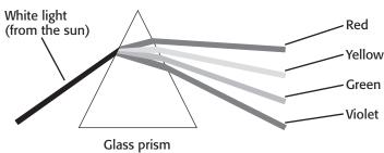
White light is separated into its component colors when it passes through a prism. The red light is refracted the least. The violet light is refracted the most.
