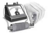
A greater electric current is induced if you move the magnet faster through the coil because the magnetic field is changing faster.
