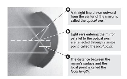
Concave mirrors can form virtual images as plane mirrors do. Concave mirrors can also form real images. A *real image* is an image that light passes through. A real image can be projected onto a screen. A virtual image cannot.
