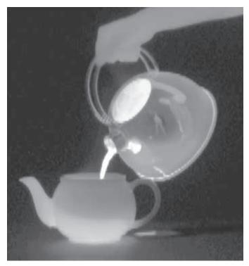
This is a photo of boiling water being poured from a kettle into a teapot. The photo was taken with a film sensitive to infrared waves. The boiling water is hotter than the hand pouring it. Therefore, the hot water is brighter in the photo.
