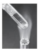
When mercury oxide is heated, it undergoes a chemical change in which it separates into the elements mercury and oxygen.
