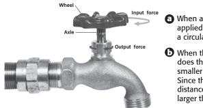
When a small input force is applied to the wheel, it turns in a circular distance.
