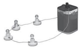
In a series circuit, the same current flows through each light bulb (load) and back to the battery.
