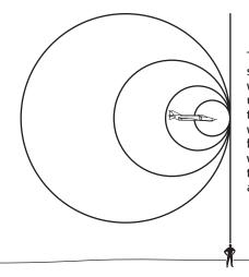
This jet is traveling at the speed of sound. The sound waves in front of the jet pile up and interfere constructively. This produces a shock wave that travels out away from the jet. When the shock wave passes the person on the ground, the person hears a sonic boom.
