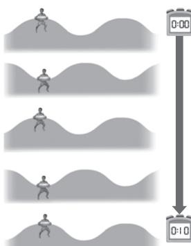
Frequency is the number of waves that pass a certain point in a given amount of time. Frequency can be measured by counting the waves that pass a certain point in a certain amount of time. In the image shown here, two waves passed by in 10 s. The frequency is 2/10 s = 0.2 l/s = 0.2 Hz.
