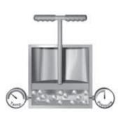
Decreasing the temperature of a gas makes the particles move more slowly. The gas particles hit the piston less often and with less force. Therefore, the volume of the gas decreases.
