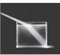
This light wave is refracted as it passes into a new medium. The light wave is passing from air into water. The wave is refracted because the speed of the wave changes.
