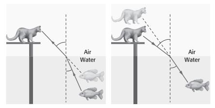
Because of refraction, the cat and the fish see optical illusions. To the cat, the fish appears closer than it really is. To the fish, the cat appears farther away than it actually is.
