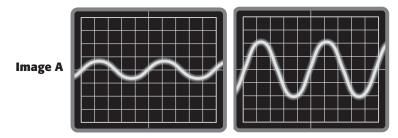
The wave in the graph on the right has a larger amplitude than the one on the left. Therefore, the sound represented by the right-hand graph is louder than the one represented by the left-hand graph.
