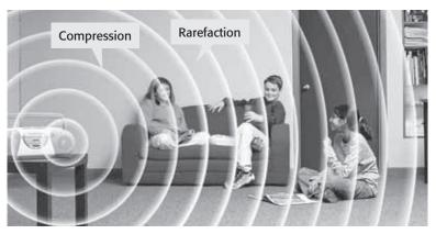
You can't see sound waves. However, they can be represented as spheres that spread out in all directions. Each sphere represents one wave (a compression and a rarefaction). In this figure, the sound waves are traveling in all directions from the radio speaker.
