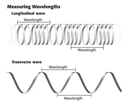
A wavelength can be measured between any two identical points on neighboring waves.
