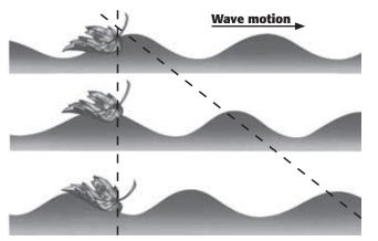
A wave travels through the medium, but the medium does not travel. In a pond, lake or ocean, the medium through which a wave travels is the water. The waves in a pond travel towards the shore. However, the water and the leaf floating on the surface only travel up and down.
