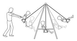
When the swing is pushed, it swings higher and higher. The amplitude of the swing increases because of pushes at the fundamental frequency of the swing.
