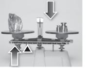
The fulcrum can be located exactly in the middle. This lever has a mechanical advantage that is equal to 1. The output force is the same as the input force.
