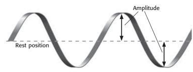
The amplitude of a transverse wave is measured from the rest position to the crest or the trough of the wave.
