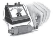
• A greater electric current is induced if you add more loops of wire. This magnet is moving at the same speed as the magnet in b.
