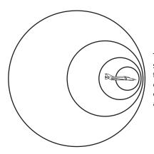
This jet is traveling near the speed of sound. The sound waves in front of the jet are pushed close together. The compression of the air particles produces an area of high pressure. This area is called the sound barrier.
