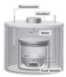
A bomb calorimeter can measure energy content in food by measuring how much heat is given off by a food sample when burned. If a food sample releases 523,000 J of heat, what is the energy content of the food? Since 1 Calorie is 4,184 J,
