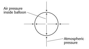
The air inside the balloon produces a pressure inside the balloon. The pressure inside the balloon equals the atmospheric pressure outside the balloon. Therefore, the balloon stays inflated.
