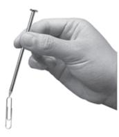
This nail was magnetized by dragging a magnet down it many times.
