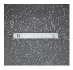
The magnetic field surrounding the magnet causes the iron filings to form arcs around it.
