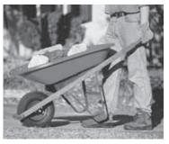
A wheelbarrow is an example of a second-class lever. Second-class levers have a mechanical advantage that is greater than 1.
